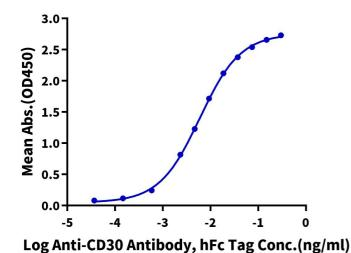
Immobilized Cynomolgus CD30, His Tag at 2µg/ml (100µl/Well) on the plate. Dose response curve for Anti-CD30 Antibody, hFc Tag with the EC50 of 6.0ng/ml determined by ELISA (QC Test).
